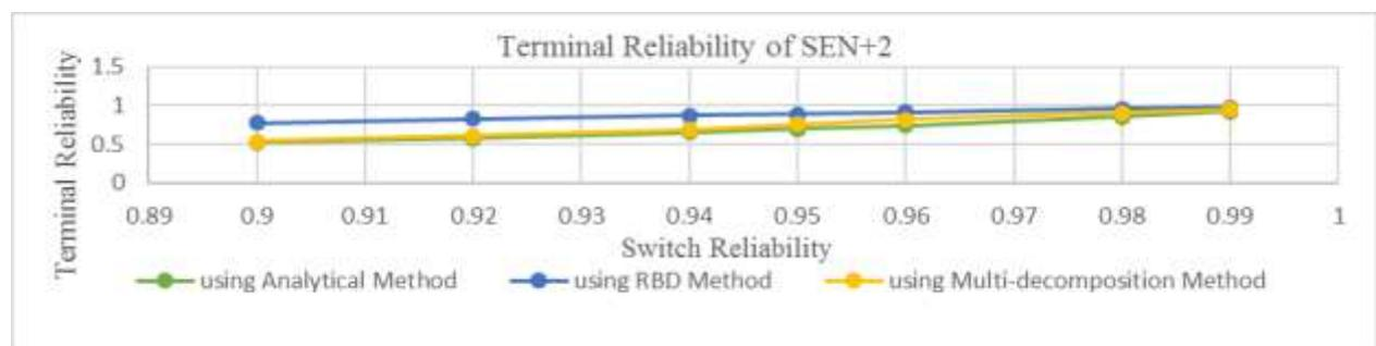
**Fig.6. Graph of Terminal Reliability of SEN+2 computed by - Analytical Method, RBD Method and Multi-decomposition Method**
